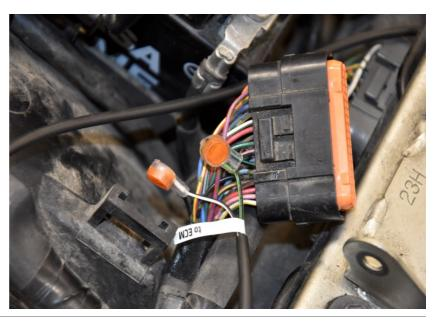
Connect the X-TRE Red wire to the Orange wire of the rear brake light switch connector.
