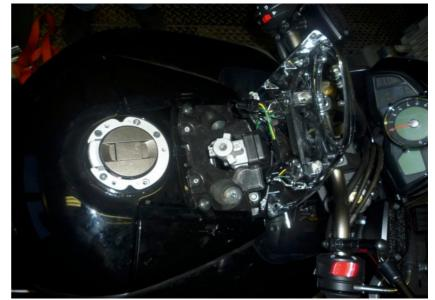
Remove the left and right black frame covers from the fuel tank.
