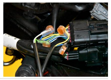
Splice the SH Red wire to the White/Green wire of the dashboard connector. Use a red wire tap connector.
