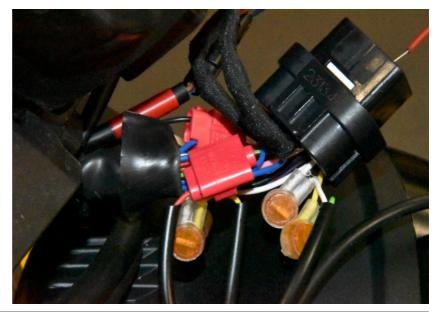
Splice the SH Black wire to the Blue wire of the dashboard connector. Use a red wire tap connector.
