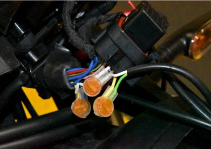
Connect the SH Yellow wire to the White wire end, which is at the wiring harness side. Use a yellow butt connector.
