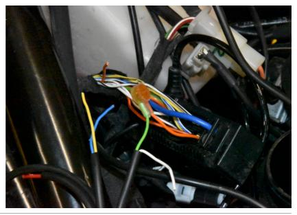
Connect the SH Blue wire to the Orange wire end, which is at the wiring harness side. Use a yellow butt connector.
