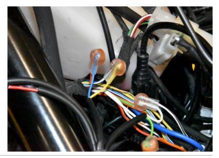
Splice the SH Red wire to the Orange/Red wire of the ABS connector. Use a red wire tap connector.
