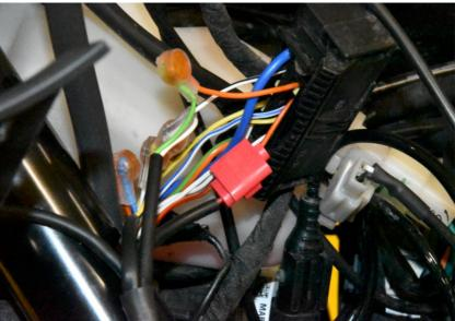
Splice the SH Black wire to the Blue wire of the grip heater connector. Use a red wire tap connector.
