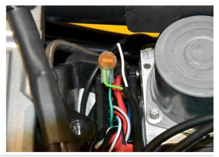
Connect the SH Blue wire to the Green/Black wire end, which is at the wiring harness side. Use a yellow butt connector.
