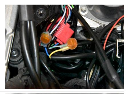
Splice the SH Red wire to the Red/Black wire of the ABS connector. Use a red wire tap connector.
