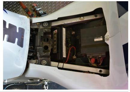
Lift up or remove the fuel tank.
