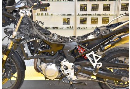
Locate the fuel injector connectors.
