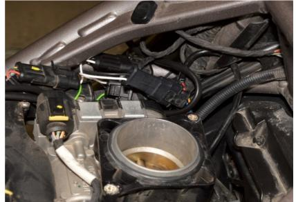
Connect the QSH connectors in-line with the ignition coil connectors on the right side.
