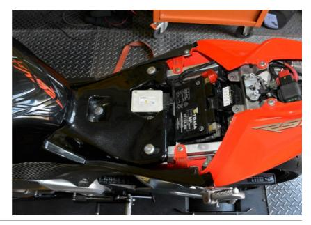
Remove the frame covers below the fuel tank.
