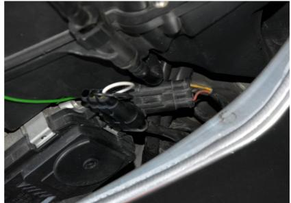
Connect the QSH connectors in-line with the ignition coil connectors on the airbox.
