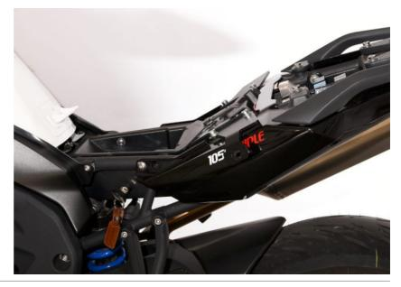
Remove the fuel tank covers and the side fairings.
