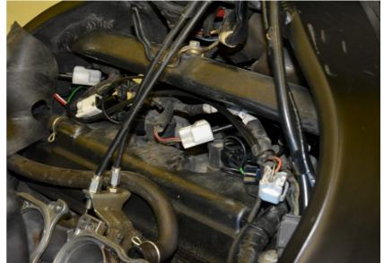
Connect the QSH Black wire terminal to the chassis ground.
