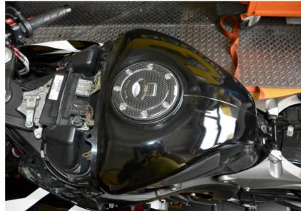
Lift up or remove the fuel tank.
