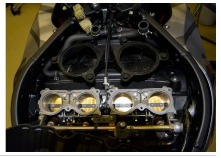
Remove the air intake below the airbox.
