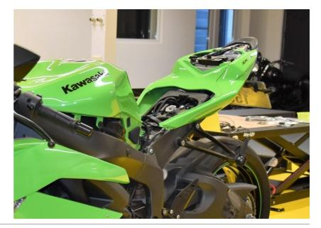
Remove or lift up the fuel tank.
