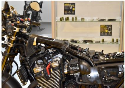
Locate the ignition coil terminals under the fuel tank.
