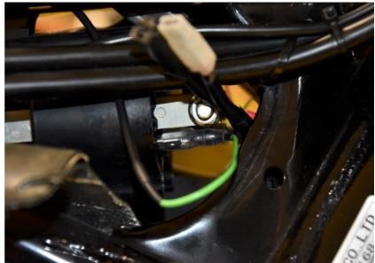
Connect the QSH Black wire terminal to the chassis ground terminal.
