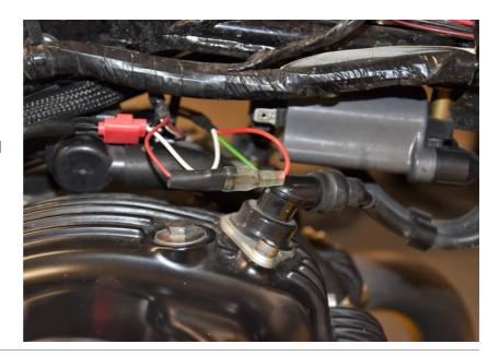
Splice the QSH White wire to the Black wire of the coil by using the supplied red wire tap connector.
