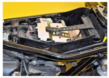
Lift up or remove the fuel tank.
