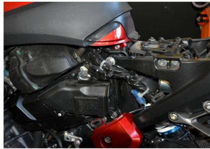
Lift up or remove the fuel tank.
