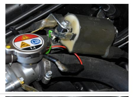
Splice the QSH White wire to the Yellow/Blue wire of the coil by using the supplied red wire tap connector.
