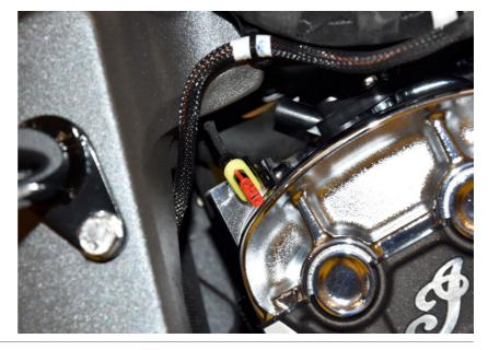
Connect the QSH connectors in-line with the ignition coil plugs.
