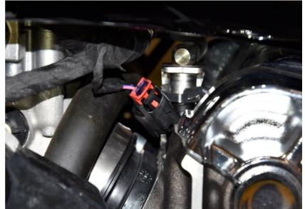
Connect the QSH White wire to the injector plug White/Blue wire.
