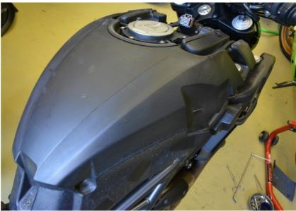
Remove or lift up the fuel tank.
