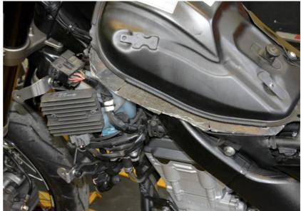
Plug the QSH connector pair which is marked with a red square in-line with the ignition coil connector.
