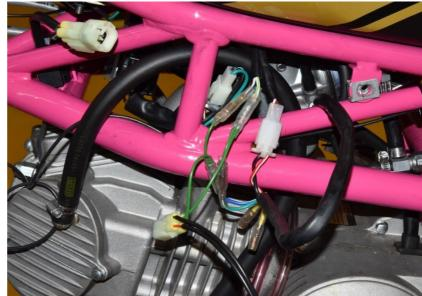
Use the supplied Black jumper wire to make a connection between the battery negative terminal and chassis ground, by placing the jumper wire terminal under the bolt of the ignition coil.
