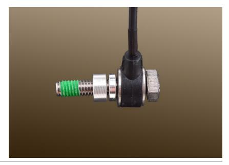
Mount the QSE sensor under the bolt of the shift lever.
