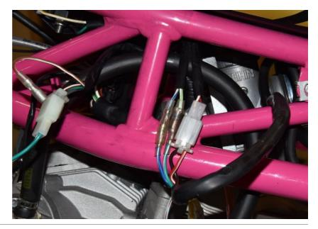
Connect the QSH Green wire terminals in-line with the 1-pole bike plugs.
