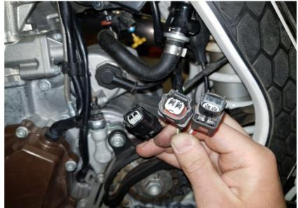
Connect the QSH connectors in-line with the injector connectors.
