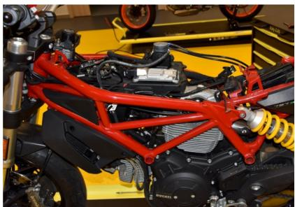
Locate the fuel injector connectors.
