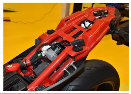
Lift up or remove the fuel tank.
