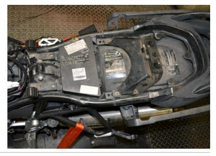
Lift up or remove the fuel tank.
