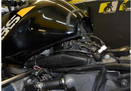
Plug the QSH connectors in-line with the fuel injector connectors.
