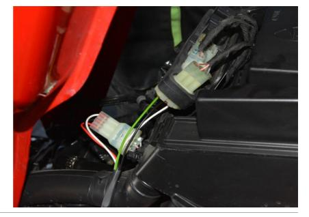
Connect the QSH Black wire terminal to the chassis ground.
