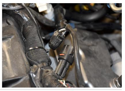
Plug the OSE connector into the wiring harness connector.
