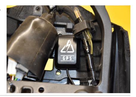
Typical position for the iLE module.
