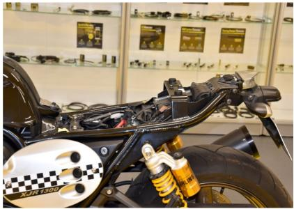
Locate the rear light assembly connector.
