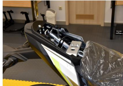
Locate the black 3-pole rear light assembly connector.
