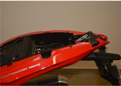
Locate the rear light assembly connector.
