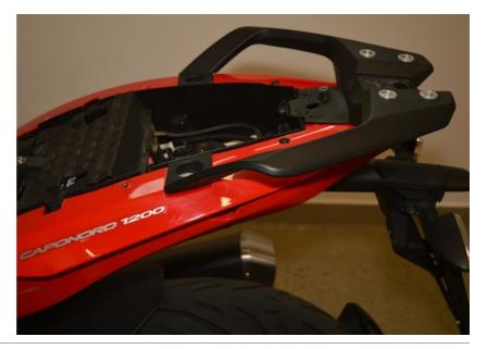
Remove the passenger handrails.
