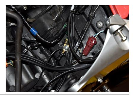
Locate the ABS ECU connectors on the left side.
