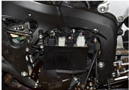
Splice the ARA Green wire to the Blue wire (pin #3) of the Gray ABS ECU connector.
