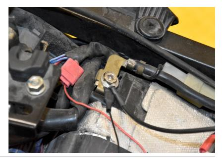
Locate the ABS connector under the right side fairing.
